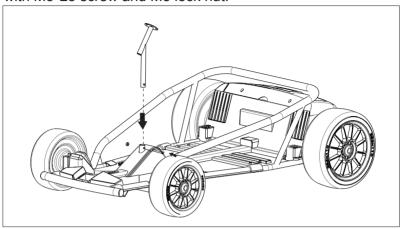
②.Insert the steering axle from the bottom to the car body and steering axle holder, until the top of the steering axle extends out the steering axle holder.
