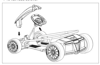
8. Seat assembly Attach the seat with seat slot on car body, fix them with 4\*16 flat head screws.
