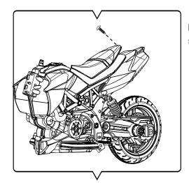
Make the screw loosen from the seat, take down the seat, then connect the battery line red wire to the red column on the battery, black wire to black part. Aoviding inserting into the uncorrect polarity. After that please put the seat on the car body again, then tighten the tapping screw and fix it properly.
