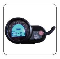
Accelerator / Switch Button/ Battery Indicator
